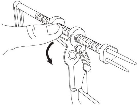
**\*Misalignment of the coring/slicing blade is the most common user mistake which will result in damage to the blade and possibly the fork.**
